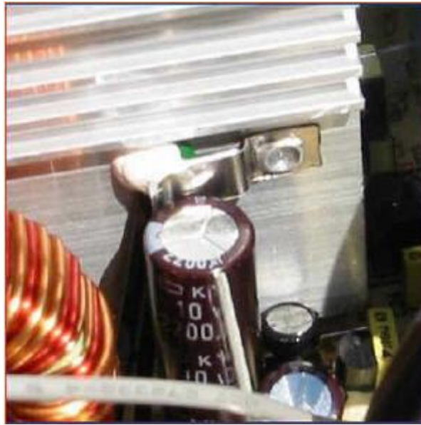
Figure 28 A thermistor protects an electronic circuit from overheating.
