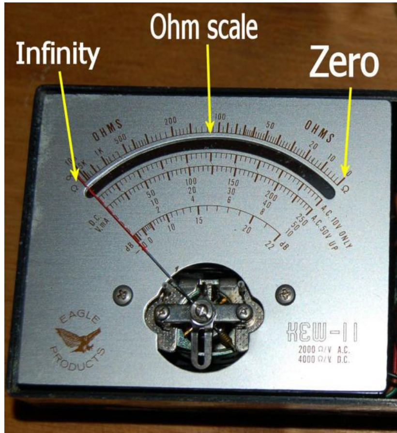
Figure 20 An analogue multimeter can be used as an ohmmeter
